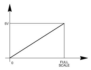
LINEAR OUTPUT, RMS CALIBRATED TO 50 or 60 Hz SINE WAVE.
