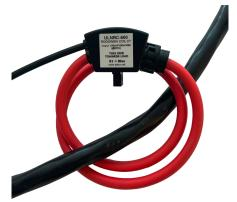
The flexible ULNRC-600 may be wrapped around the primary conductor multiple times for tighter installation, higher input sensitivity and accuracy.
